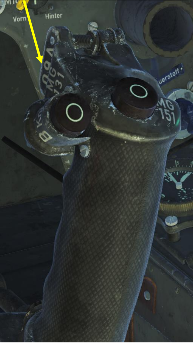
A Button Inner Wing MG 151 Cannon & MG 131 Machinegun Button • Note: If the Cannon Safety Cover is ON, the MG 151/131 Trigger will only fire machineguns when pressed.
