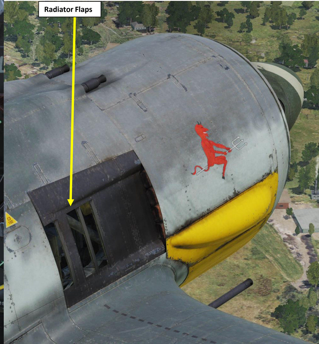
Radiator Flaps Position Indicator • Up: Zu (Closed) • Down: Auf (Open)
